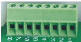
1. Power supply 24 V AC/DC, 100 mA (polarity is not important)
