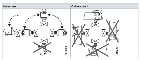
1) Requires the weather shield ASK39.2. Degree of protection of housing IP54 remains unchanged.
